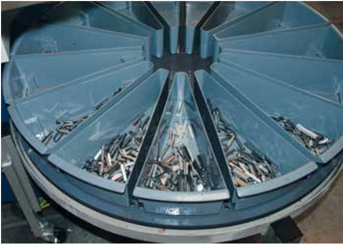
Performance Design's parts carousel with fifteen bins holds a complete Rhin-o-Tuff pin set (a pin set is the same pin in fifteen lengths).
