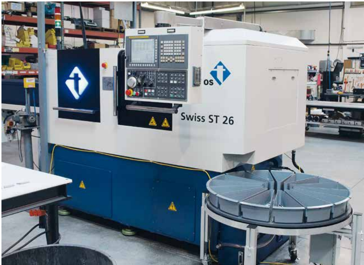
Swiss ST 26 with parts carousel shown.
