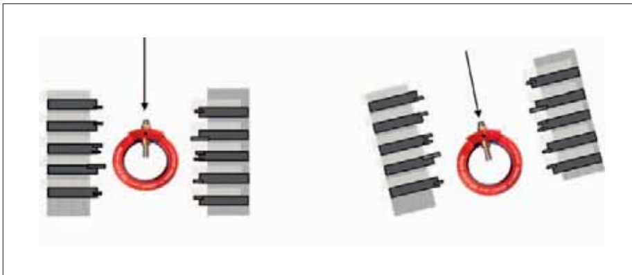
Fitting on the guide bush. The vertical axis of the sensor must be positioned along the same plane as the vertical axis moving the platters.
