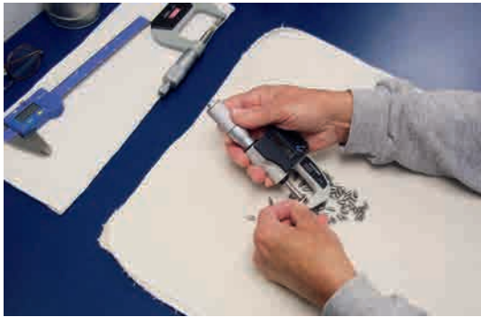
Quality Control engineers using a digital micrometer to check tight tolerances for a part made in one of the SwissNanos.
