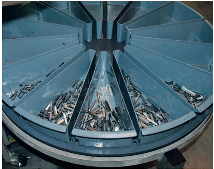
Performance Design's parts carousel with fifteen bins holds a complete Rhin-o-Tuff pin set (a pin set is the same pin in fifteen lengths).
