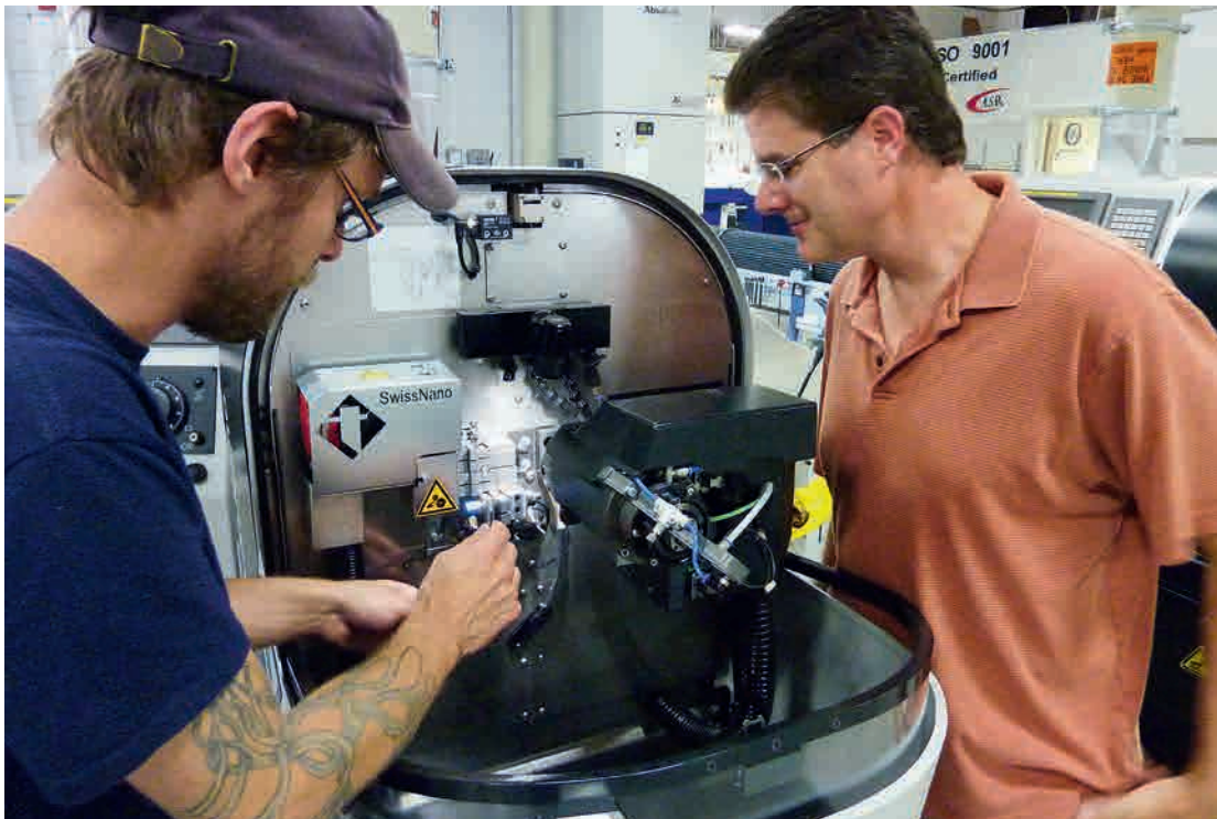
Petron’s CNC Manager and Plant Manager fixing a 7-degree angle block in one of the new SwissNanos to manufacture a customer part for the Medical and Electronics industries.
